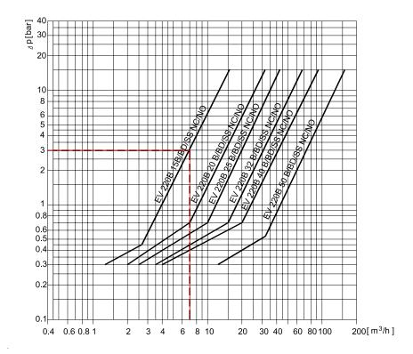
Example, air: Capacity for EV220B 15B at inlet pressure ( $p^1$ ) of 5 bar and outlet pressure ( $p_2$ ) of 3.5 bar: Approx. 245 Nm<sup>3</sup>/h
