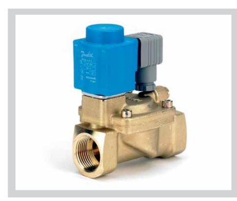
EV220B 15–50 is a universal indirect servo-operated 2/2-way solenoid valve program. Valve body in brass, dezincification resistant brass and stainless steel ensures that a broad variety of application can be covered.
